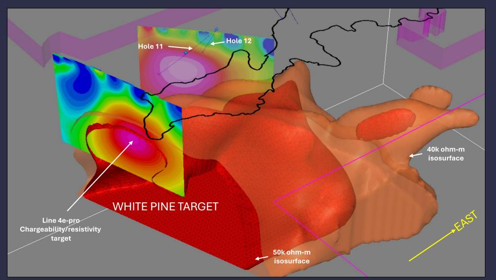
The Line 4E pro section shows coincident high resistivity and chargeability. This is a similar signature to the Red Cedar Discovery – therefore, this is a prime drill target.
